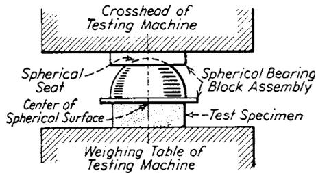
**FIG. 1 Spherical Bearing Block for Compressive Strength Test**
