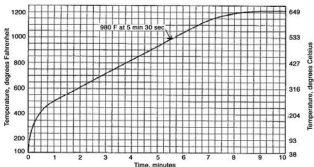
FIG. 8 Representative Time-Temperature Curve for Red Oak
