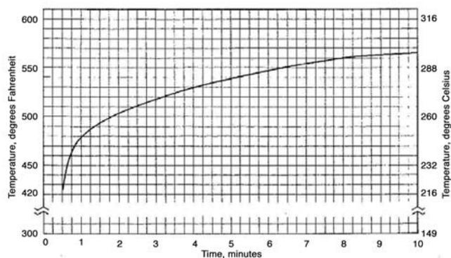
FIG. 6 Representative Time-Temperature Curve for Preheat Temperatures
