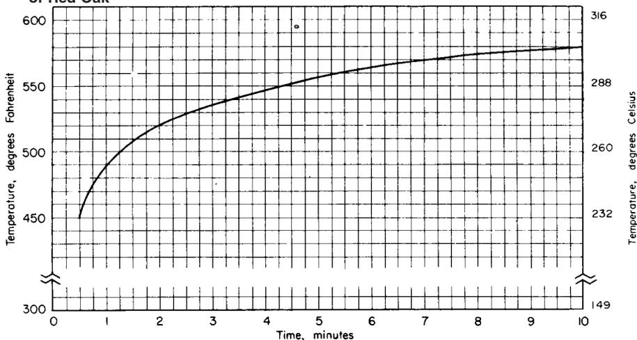
FIG. 10 Representative Time-Temperature Curve for Fuel Contribution of Fiber-Cement Board
