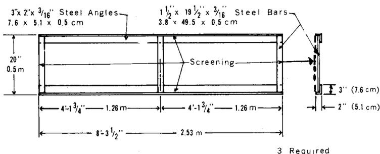
**FIG. X1.2 Steel Frame for Loose Fill Insulation**
